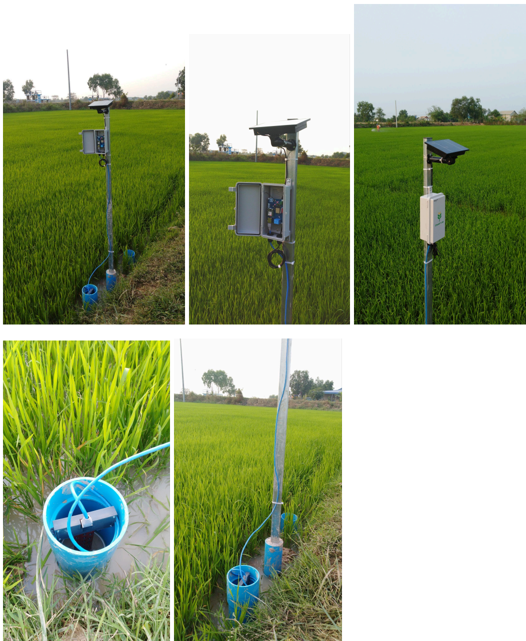
Figure 3.3: Chalate Tube Sensor Installed in the rice field located at Bati District, Takeo Province, Cambodia (07/04/2025)
