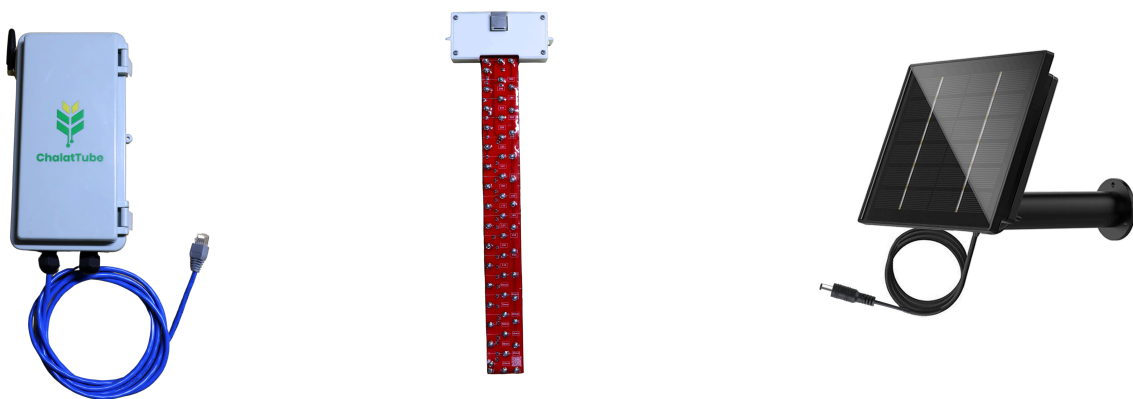
Figure 1.2: Chalat Tube Water Rice Field Water Level Sensor (v4.0). Fully assembled sensor PCB housing inside plastic enclosure (left) 30 30-channel analog-based water level sensor (middle), solar panel with built-in battery pack (right)
